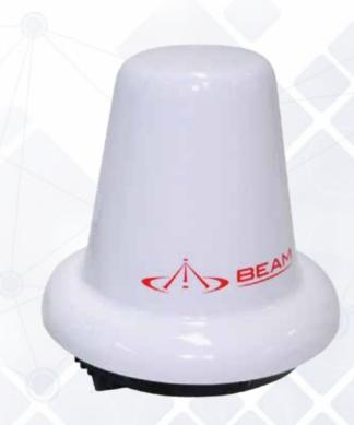
Where an installation exceeds 20m/60ft it becomes more cost effective to use an Active/Powered Iridium antenna that allows much thinner and cheaper cable to run up to 100m/300ft where this would never be possible with a passive Iridium antenna. The Active Antenna RST740 will work on all Beam products and any Iridium devices, however requires an approved Beam Active Antenna cable for use in order to manage the power amplification across the RF line to the antenna.
